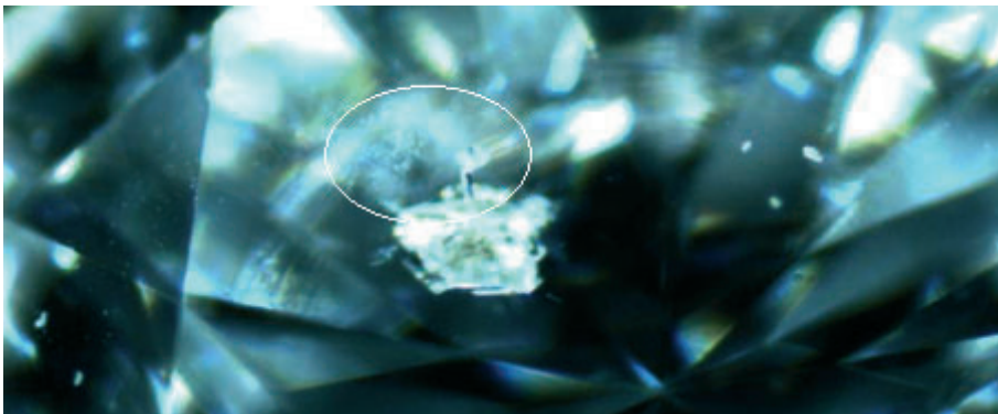
Laser drilled with burn on entry facet
